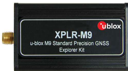
Figure 1: Explorer kit (60 x 32 x 15 mm)
