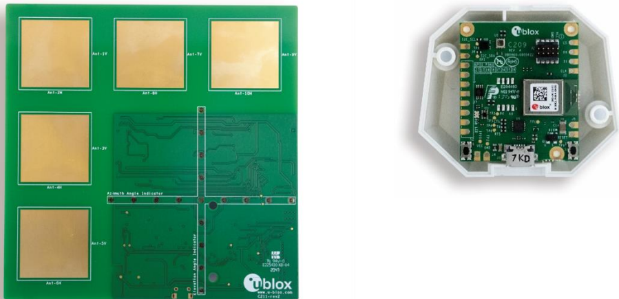
Figure 1: u-blox direction-finding explorer kits comprising C211 application board(s) and C209 tag(s)
