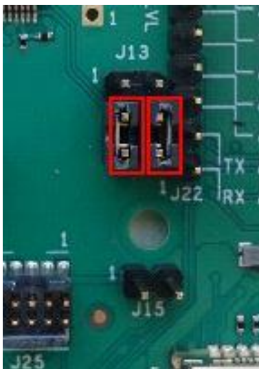
Figure 11: UART selection jumpers to be removed on ODIN-W2 EVK
