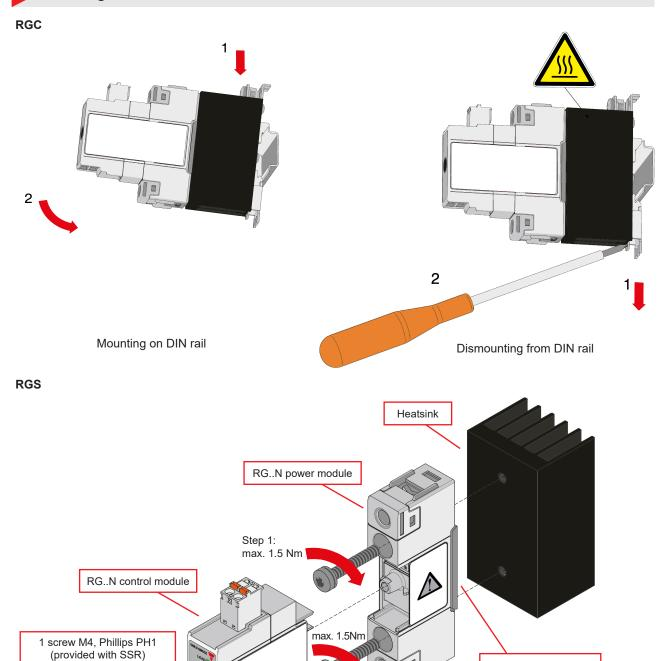
Step 1: Mount RG..N power module to Heatsink
