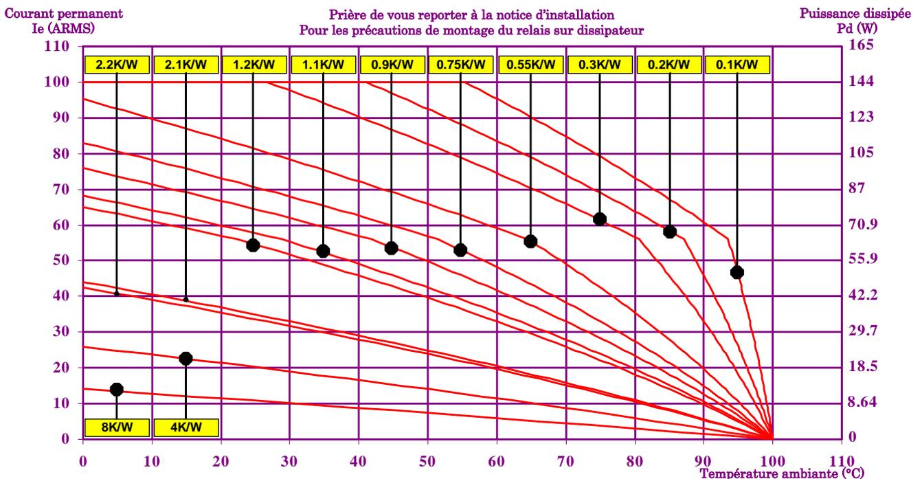
10K/W = Sans dissipateur / 1LD12020      4K/W = Plaque d'aluminium de 150x150x3mm      2.2K/W = WF262100 / WF151200      2.1K/W = WF21000
