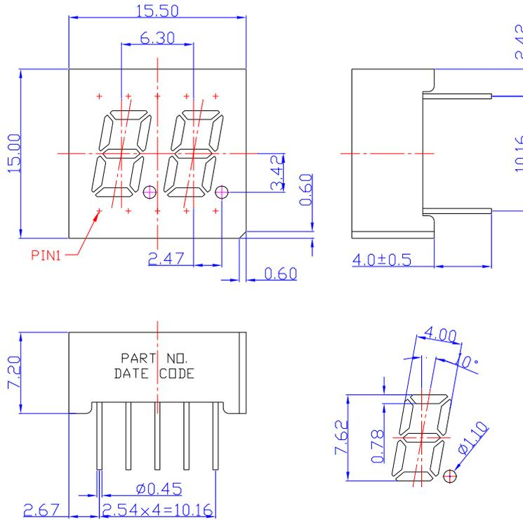
NOTES: Dimension is in millimeters. Tolerance is  $\pm 0.25$  mm unless otherwise noted.
