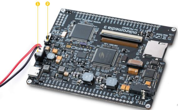
Figure 8: Battery power supply connection
