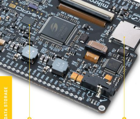
Figure 10: MicroSD card slot view
