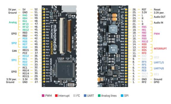
Figure 13: 1x26 pin header view
