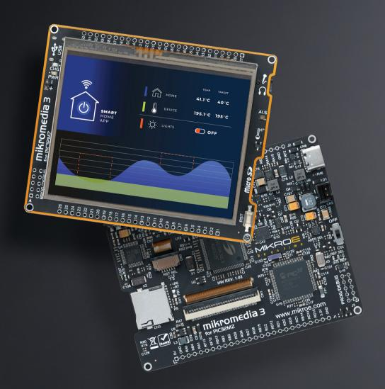
mikromedia 3 for PIC32MZ RESISTIVE is a compact development board designed as a complete solution for the rapid development of multimedia and GUI-centric applications. By featuring a 3.5" resistive touch screen driven by the powerful graphics controller that can display the 24-bit color palette [16.7 million colors], along with a DSP-powered embedded sound CODEC IC, represents a perfect solution for any type of multimedia application.
