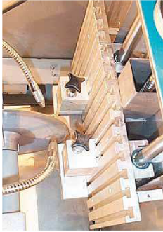
drylin® R linear plain bearings on supported aluminum shafts are used in this grinder to guide the cutting table. The drylin® components stand for extrema dirt resistance, accurate guidance and smooth operation.
