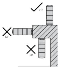
Choose a flat surface with enough strength and with little vibration for installation. Mount this product according to the figure to maintain IP characteristics of the figure to maintain IP characteristics. NO
