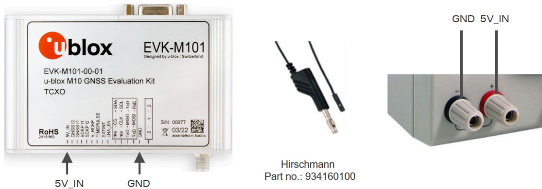
Figure 3: EVK-M101/C 5.0 V DC power supply example
