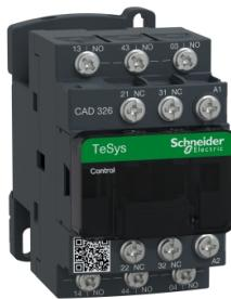
TeSys D control relay - 3 NO + 2 NC - <= 690 V - 24 V AC standard coil
