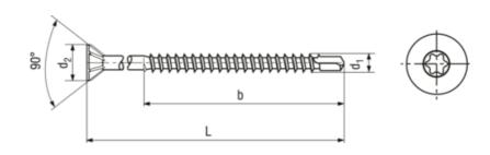
Headform Countersunk with cutting ribs
