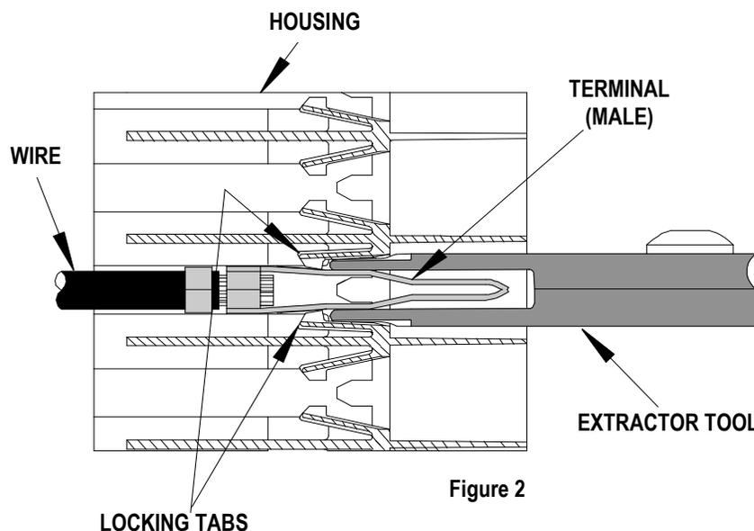
**CAUTION:** This extractor tool should be used to extract the terminal only. Using it for unintended purposes may cause injury or damage to parts. Be careful not to deform the end of the terminal. Avoid lifting the housing lock too high.
