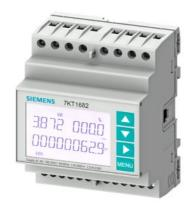
SENTRON, measuring device, 7KT PAC1600, LCD, L-L: 400 V, L-N: 230 V, 5 A, strd rail instr., 3-phase, Modbus RTU/ASCII, power monitoring incl. THD, AC/DC, screw terminals
