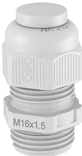
The quickest and most convenient way of providing strain relief and tightness with cable glands on junction boxes and housings is with the tried-and-trusted V-TEC VM cable glands from OBO. A protection rating of IP68 is achieved through the integrated sealing lip and the special OBO slat technology. Strain relief and tightness have been tested to DIN EN 62444.
