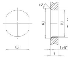
Installation direction: o-ring sits on chamfer.
